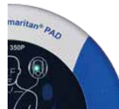
Figure 10. Flashing green LED; no action required.
